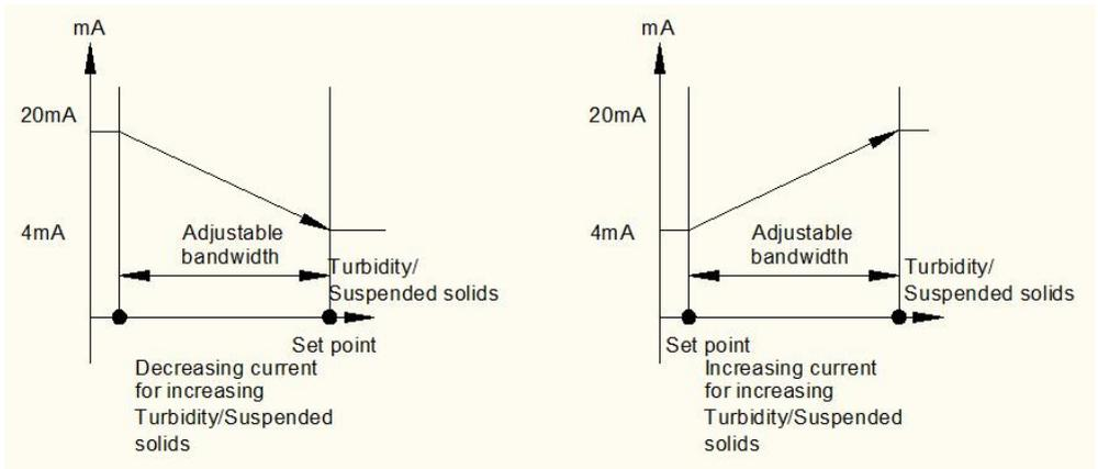
The analog output will produce a linear analog output if the user selects this option. The analog output will be dependent on the Turbidity or Suspended Solids\_4 mA setting, Turbidity or Suspended Solids\_20 mA setting and the current Turbidity or Suspended Solids display.
