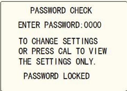
A screenshot of a monochrome LCD screen with a yellow background. The text is centered and reads: "PASSWORD CHECK", "ENTER PASSWORD: 0000", "TO CHANGE SETTINGS OR PRESS CAL TO VIEW THE SETTINGS ONLY.", and "PASSWORD LOCKED".
