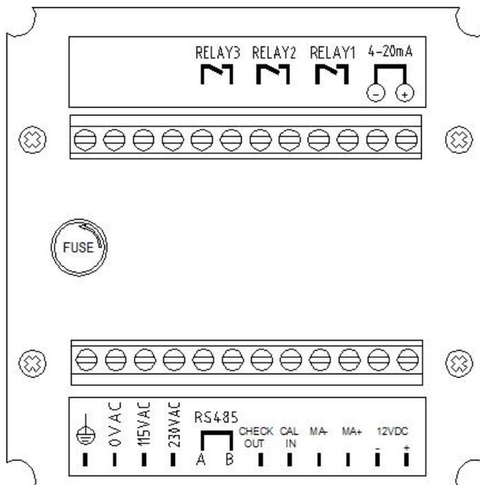
Before connecting the probes, relays, analog output, RS485 and power cord be sure that you are connecting to the right terminal as shown above. Remember that the unit is on once the user plugs in the power cord to an AC power supply.
