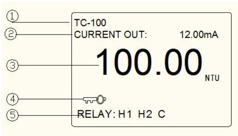
1. **TC-100** annunciator- this is the sensor selection mode. The model 6308TuSS can work with 5 different 5 sensors, they are: TC-100、 TC-500、 TC-3000、 TCS-1000 and TS-MXS-A.
