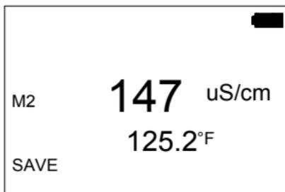
**Note:** The Model pH/EC 80 is equipped with a non-volatile memory that can store up to 50 different sets of readings (pH/Conductivity/TDS/Salinity and temperature). Non-volatile memory will be retained even if power is lost. When all 50 memory locations are used up, the next set of data saved will overwrite the data stored in the first location and so on.
