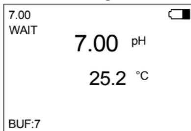
3. When the “WAIT” icon disappears, one point/first point calibration is now complete. Press “Mode” key to exit or to wait 5 seconds for the meter to enter two points / second point calibration.
