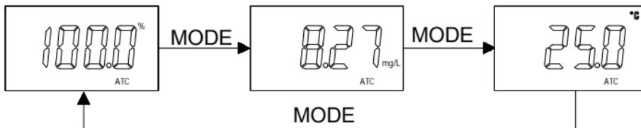
1. **DO(%)** –A measurement of oxygen in percent saturation.
