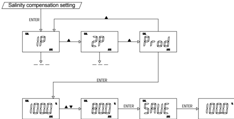
Press the **[UP]** or **[DOWN]** key to change the value to your specified value. Then press the **[ENTER]** key to save your product calibration and the unit will automatically move to the **“Measure mode”**.
