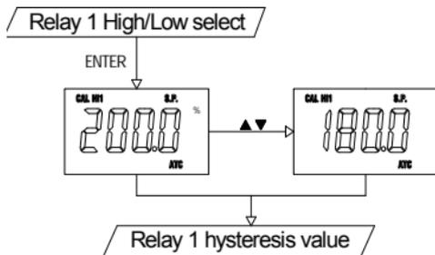
Pressing **[UP]** key or **[DOWN]** key in this screen to adjust the value, press **[ENTER]** key to save, and enter the next setting screen.
