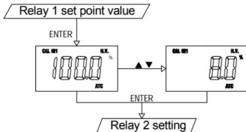
Pressing **[UP]** key or **[DOWN]** key in this screen to adjust the value, press **[ENTER]** key to save, and enter the next setting screen.
