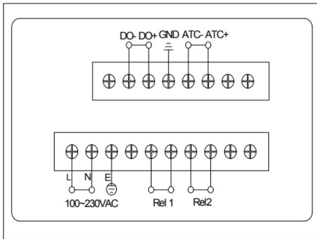
1. Connect the AC line to the rear of the instrument. The model 3921 can be used with 100~240V AC at 50/60 HZ. Make sure the **EARTH** connector is connected to the earth lead of the AC power line.
