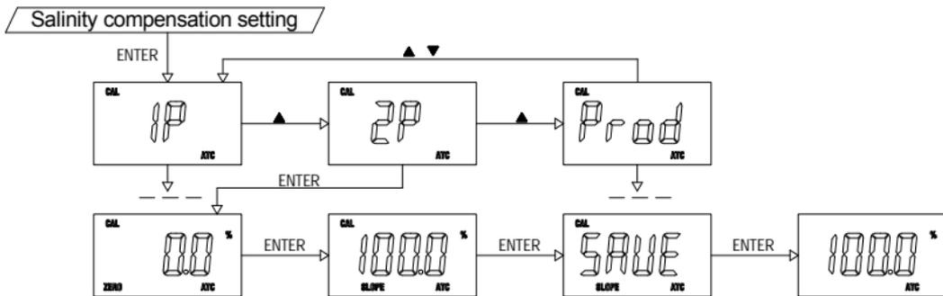
Press the [**UP**] or [**DOWN**] key to select “**2P**” then press the [**ENTER**] key to save the selection, the unit will automatically move the “**ZERO calibration**”.
