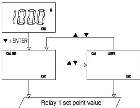
Pressing [**UP**] key or [**DOWN**] key in this screen will cycle the display from HI1 、 LOW1 modes above. Select the preferred mode, press [**ENTER**] key to save, and enter the next setting screen.
