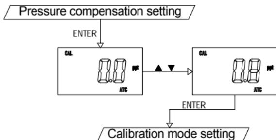
compensation factor, use the **[UP]** key or **[DOWN]** key to adjust the value between 0.0 and 49.9ppt. Press **[ENTER]** to save the new value and the unit will automatically go into the next calibration parameter.
