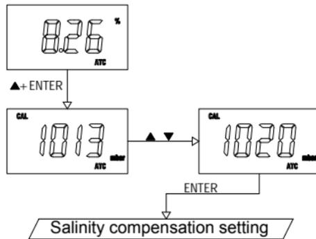
In the **DO measure mode**, pressing **[UP]** key and **[ENTER]** key at the same time to allow the meter to go to the **pressure compensation setting**. The main screen will display “1013mbar” (factory default value). To change the pressure factor, press the **[UP]** or **[DOWN]** key to adjust the value between 600 and 4000mbar. Press **[ENTER]** to save the new value and the unit will automatically go into the next calibration parameter.
