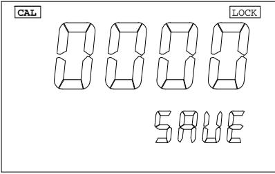
This screen selects the password number for this unit. The user can use [ $\blacktriangle$ ], [ $\blacktriangledown$ ] or [ $\blacktriangleright$ ] keys to input the new password. Pressing the [OK] key will save the password number and LOCKS the unit. You will not be able change any setting or turn-on
