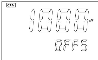
This screen selects the OFFSET for relative ORP. The value here will be subtracted from the absolute ORP reading to display the relative ORP reading. The equation is :
