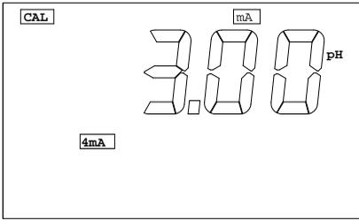
This screen will let the user change the 4 mA value. The user can use [ $\blacktriangle$ ], [ $\blacktriangledown$ ], [ $\blacktriangleright$ ] or [**OK**] keys to input new 4mA value. This value is used for scaling the 4-20mA **ANALOG OUTPUT**. (For detailed explanation see chapter **VI. 4-20 mA OUTPUT**.)
