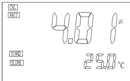
After finishing the Buffer I calibration the unit will move to this screen. The initial display will be the chosen buffer for **pH BUFFER II SELECT**. The "SLOPE" annunciator will blink indicating that the unit is waiting for the user to continue the calibration. Put the
