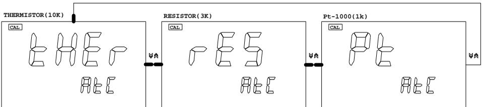
This screen will let the user select what temperature probe (10K $\Omega$  thermistor, Balco 3K $\Omega$  resistor or RTD pt-1000) the user will use. This screen will always default to the last temperature probe the user selected. For most application the user will only use one kind of
