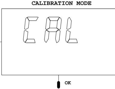
Pressing the [OK] key at the CAL mode will bring-up the PASSWORD CHECK display if the unit is LOCKED. If the unit is not locked, the unit will skip the PASSWORD CHECK screen and go directly to CALIBRATION SELECT screen.
