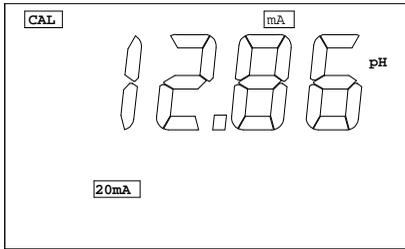
This screen will let the user change the 20 mA value. The user can use [ $\blacktriangle$ ], [ $\blacktriangledown$ ], [ $\blacktriangleright$ ] or [**OK**] keys to input new 20mA value. This value is used for scaling the 4-20mA **ANALOG OUTPUT**. (For detailed explanation see chapter **VI. 4-20 mA OUTPUT**.)
