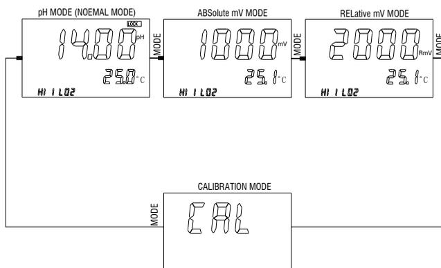
Turning ON the unit will always display **MAIN** display mode.
