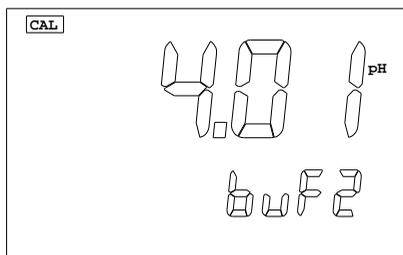
This screen selects the buffer for slope calibration. The user can select "1.68pH", "4.00pH", "4.01pH", "9.18pH", "10.01pH" or "12.46pH". Press the [▲] or [▼] keys to select the buffer then the [OK] key to save your selection. The next two steps
