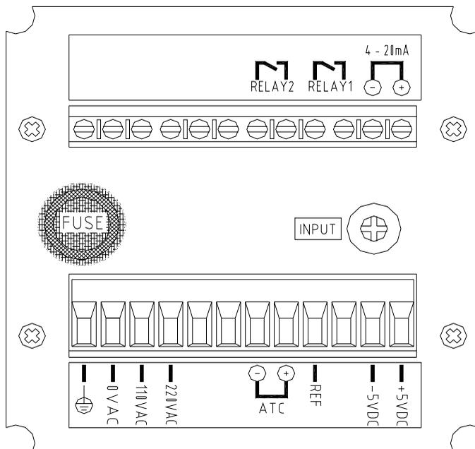
Before connecting the probes, relays, analog output and power cord be sure that you are inserting to the right terminal as shown above. Remember that the unit is ON once the user plugs in the power cord to an AC power supply.
