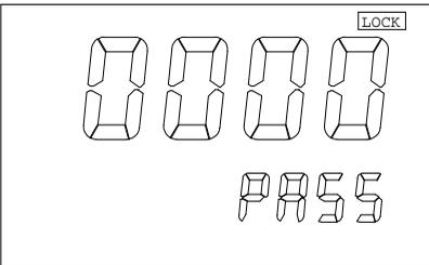
You will only see this screen if the unit is LOCKED. To change any settings or calibration you need to unlock the system to remove the "LOCK" message. You can use [▲], [▼], [▶] or [OK] keys to enter the correct 4-digit number on the
