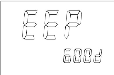
After the unit is turned on, the unit will display the software version number ("Ver"=Version) then it will perform some basic self-diagnostics ("EEP" = EEPROM Check, "RO-" = ROM Check & "RA-" = RAM Check) and will display "GOOd" or "bAd".
