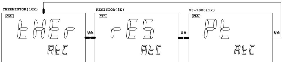
This screen will let the user select what temperature probe (10KΩ thermistor, Balco 3KΩ resistor or RTD pt-1000) the user will use. This screen will always default to the last temperature probe the user
