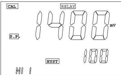
This screen is essentially the same for the two relays. Take note of the blinking character as there are 3 values to input for each relay. The user can use [ $\blacktriangle$ ], [ $\blacktriangledown$ ], [ $\blacktriangleright$ ] or [OK] keys to input the SET-POINT first then the HYSTERISIS and finally
