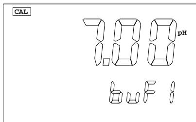
This screen selects the buffer for standardization calibration. The user can select "7.00pH" or "6.86pH". Press the [▲] or [▼] keys to select the buffer then the [OK] key to save your selection.
