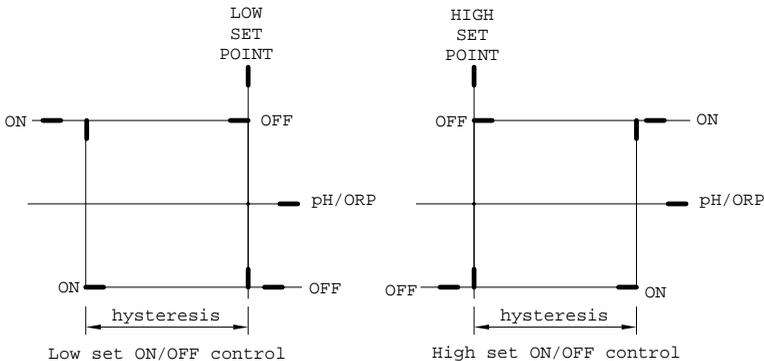
The figure above shows how the relays react to user set point, hysteresis and reading.
