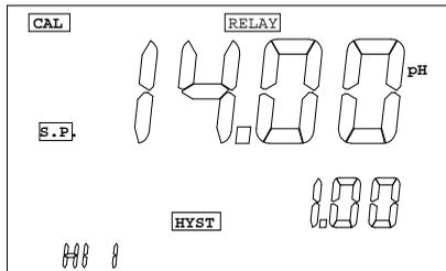
This screen is essentially the same for the two relays. Take note of the blinking character as there are 3 values to input for each relay. The user can use [ $\blacktriangle$ ], [ $\blacktriangledown$ ], [ $\blacktriangleright$ ] or [**OK**] keys to input the **SET-POINT** then the **HYSTERISIS** and finally the **RELAY ACTION**. (See **V. CONTROLLING THE RELAYS**.)
