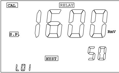
This screen is essentially the same for the two relays. Take note of the blinking character as there are 3 values to input for each relay. The user has to input the **SET-POINT** first then the **HYSTERISIS** and finally the **RELAY ACTION**.
