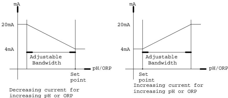
The above figure shows the relationship between Reading,  $U_{4mA}$  &  $U_{20mA}$ .
