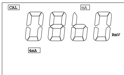
This screen will let the user change the 4 mA value. This value is used for scaling the 4-20mA ANALOG OUTPUT.
