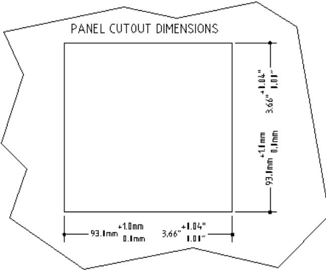
1. Make a cutout on any panel, with a thickness of **1/16 in. (1.5 mm) to 3/8 in. (9.5mm)**.
